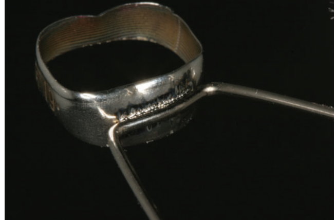
Figure 6 Band-to-wire joints. Band material: Dura-Fit (Forestadent, Pforzheim, Germany)
