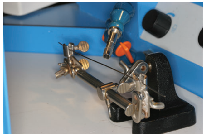
Figure 7 Standardized stabilization for brazing or welding
